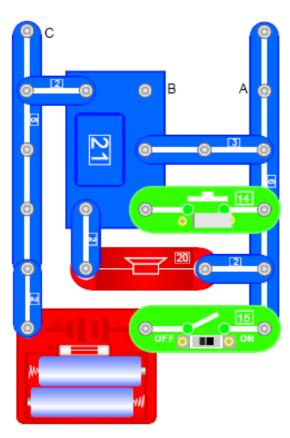
The next section of experiments all feature module 21. This is a sound module using a multi vibrator integrated circuit to produce a musical tune. All the experiments start with the circuit shown.
