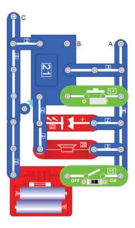
In the following experiments 84 to 94, an LED is included in the circuit to give a visual indication that the doorbell is sounding. This would be useful for the hard of hearing.
