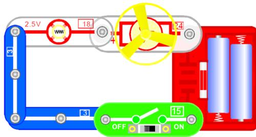
Do not connect anything directly across the battery terminals. If this happens the fuse will blow and will have to be replaced. A blown fuse is shown by a red LED on the battery holder.
