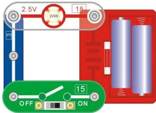
Clip the battery holder and the blue 3 connector to the base-board then clip the lamp holder and switch as shown. Be careful not to clip anything directly across the battery terminals.
